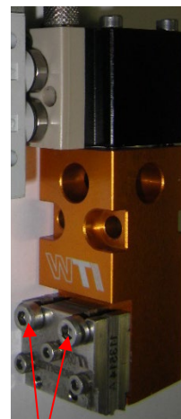
UFD High-Speed Nozzle's two mounting screws
