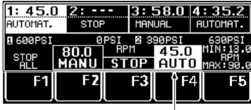
AUTO Mode is selected for Pump #1, speed is 45.0 RPM
